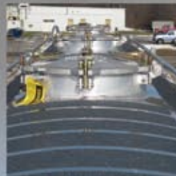
Manholes - Toe Rails
